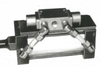
The precision automatic single measuring valve delivers fluids at an adjustable output of 0 to 40 oz. per stroke. Nozzle, hose and stylist can be tailored to suit any special applications. Proportioning piston is driven by a conventional supply pump.
